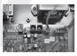
Each touch screen control is to be wired to the Aquamaster Control Box. The maximum cable length from the touch screen control to the Aquamaster Control Box is 50 meters. Recommended minimum cable size is 24AWG (7/020) or Category 5 shielded data cable.
