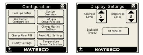
The user may adjust screen settings of Contrast Level and Brightness Level by selecting the relevant icon up and down arrows to the desired display setting. The backlight timeout may also be adjusted by pressing the relevant icon until the desired timeout is selected.
