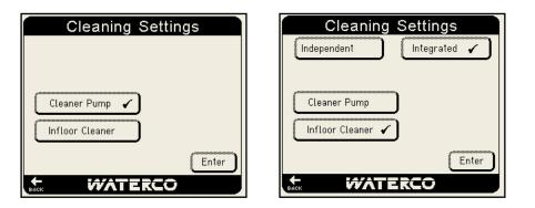
If the installed system is fitted with a Cleaner Pump select the "Cleaner Pump" icon and press "Enter".
