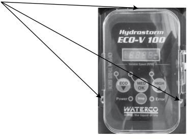
Step 2 - Lift the control housing off the pump to reveal the motor control box.
