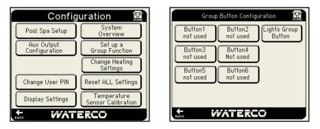
To program a group button press any icon showing "not used". On the next screen press the icon "Edit Group Button" which allows the programmer to select from installed equipment a pre programmed sequence of multiple functions operated from one named icon.
