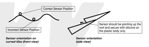
The sensor should be orientated such that it lies on the crest of the roof tiles and not in the troughs. This eliminates water being trapped in the silicon glue that holds the sensor in place, and giving erroneous readings. The roof sensor should also be positioned so that it points up the roof tiles (as shown above).
