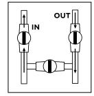
When your valves position are as shown on Figure 2, the water is going through the pool heat pump.
