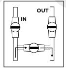
When your valves position are as shown on Figure 1, the water is bypassing the pool heat pump.
