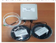
The Kit 13 Dual Heater Interface (8519128) is designed to be connected to the Pooltek unit and switch between 2 heating sources (Gas Heater & Heat Pump) where the Heat Pump is utilised for heating the pool and the Gas Heater is utilised for heating the spa. The Gas Heater can also be over-ridden to heat the pool.
