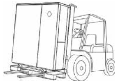
The heat pump is supplied mounted to a pallet. Once transported to site, remove the screws securing the pallet to the unit to install on the prepared slab / brackets.
