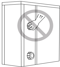
Do not lift the water union as you may damage the heat exchanger
